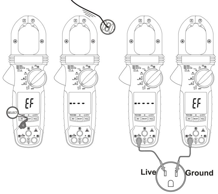
•Non-Contact EF-Detection: An antenna is located along the top-right end of the stationary clamp jaw, which detects electric field surrounds energized conductors. It is ideal for tracing live wiring connections, locating wiring breakage and to distinguish between live or earth connections.
