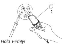
L LED indicates that the field is rotating towards the left direction of the "probe -". With this connection, the motor will go negative rotation.
