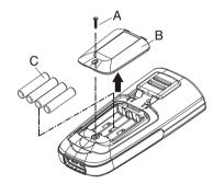
A. Screw B. Battery Cover C. Battery
