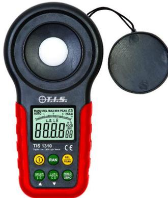
1. **Power On** by pressing the yellow power button in the top left corner. The TIS 1310 will default to normal Lux / Auto setting.
