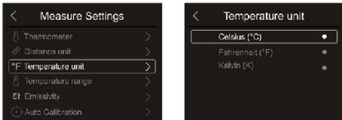
Fig. 26: Menu Setting the temperature measuring unit
