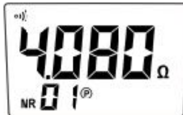
Fig. 29: Recalling result to the display
