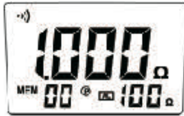
Fig. 27: Saving the result of a resistance measurement in the memory
