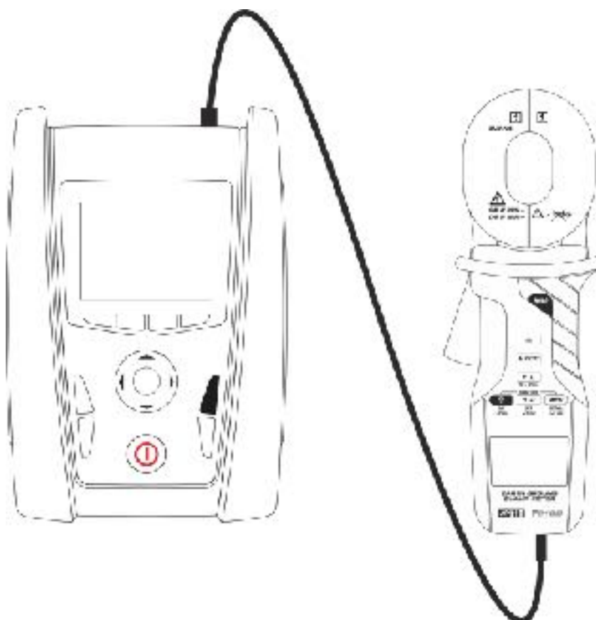
Fig. 34: Connecting T2100 to a MASTER instrument
