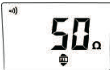
Fig. 33: Setting of alarm thresholds in resistance measurement
