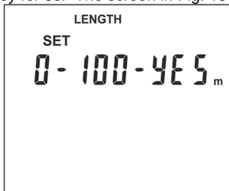
Fig. 15: Calibration settings of cable length
