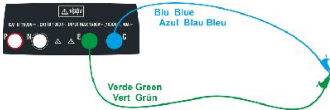
Fig. 5: Compensation of the measuring cables resistance
