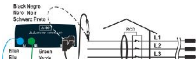
Fig. 23: Connection for three-phase L1-L2-L3-N (no PE) system by means of single cables and remote switch probe
