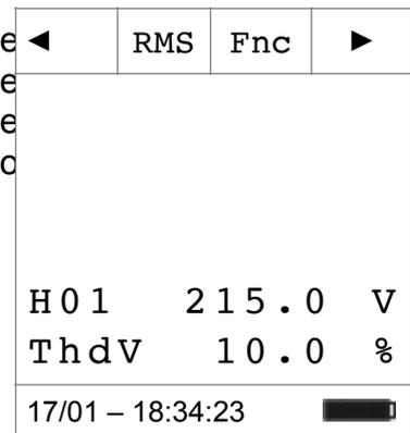
3. While measuring Voltage Harmonics, press **F3 (Fnc)** to open the display menu and select the measurement mode. At each
