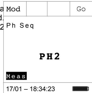
9. If the two phases, to which the test lead has been connected, are in the correct sequence, the message "**123**" is displayed. If the phase sequence is incorrect, the message "**132**" is displayed
