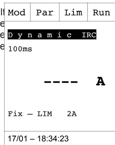
11. Press **F4 (Run)** to start a new measurement or move the selector to exit from the function
