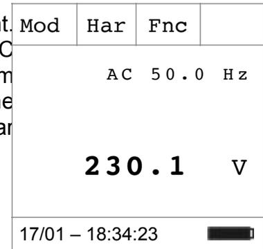
6. Press **F3 (Fnc)** to open the drop-down menu shown on the screen aside. At each subsequent pressure of key **F3**, the cursor will scroll through the available items, as follows:
