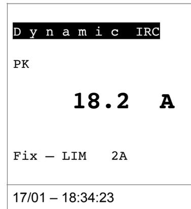
10. Press the **F4 (Sav)** key to save the measurement result within the IRC memory (see § 4.4.6). It is possible to save up to 20 IRC measurements in the memory. Then the message "MEM FULL" is shown in the lower part of the display
