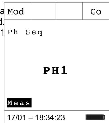
6. Once phase L1 acquisition is complete, the instrument stops the acoustic signal and the “**Discon.**” Message is shown. Disconnect the test lead from phase L1 cable.
