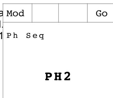
7. If there is correct conformity between the two phases, to which the test lead has been connected, the message “11-” is displayed. If not, the messages “123” or “132” are displayed.
