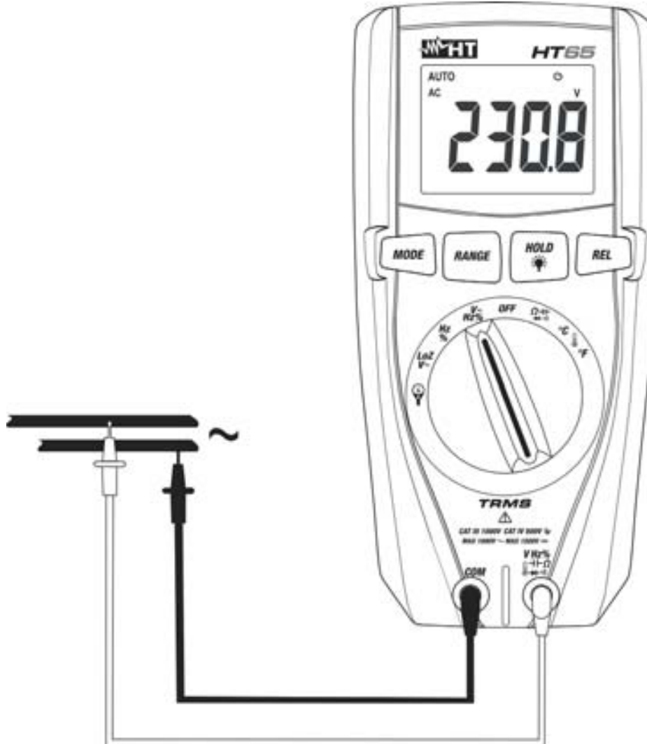
Fig. 3: Use of the instrument for AC voltage measurement
